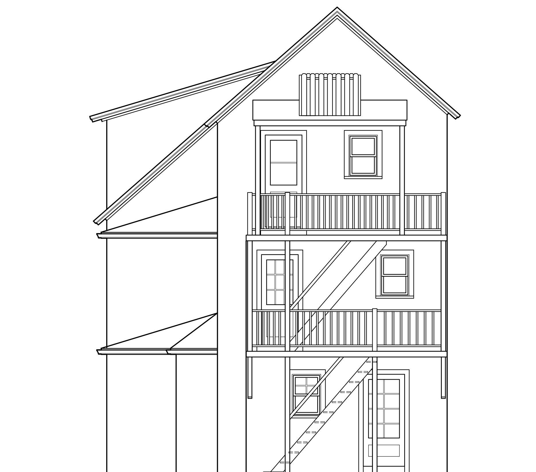
1 EXISTING REAR ELEVATION V-3 SCALE: 1/4" = 1'-0"
